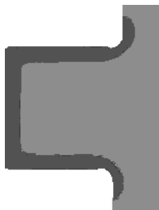
Raceways of a nose ring in a three-row roller bearing slewing
