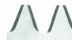
齿面淬火 Tooth face quenching
