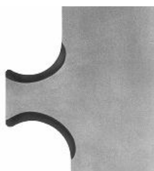
Raceways of a nose ring in a double-row ball bearing
