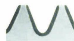
齿面齿根淬火 Tooth face and tooth root quenching
