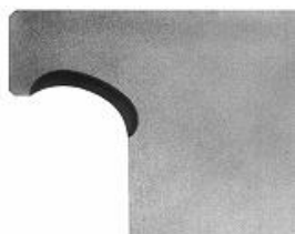
Raceway of a supporting ring in a double-row ball bearing slewing ring
